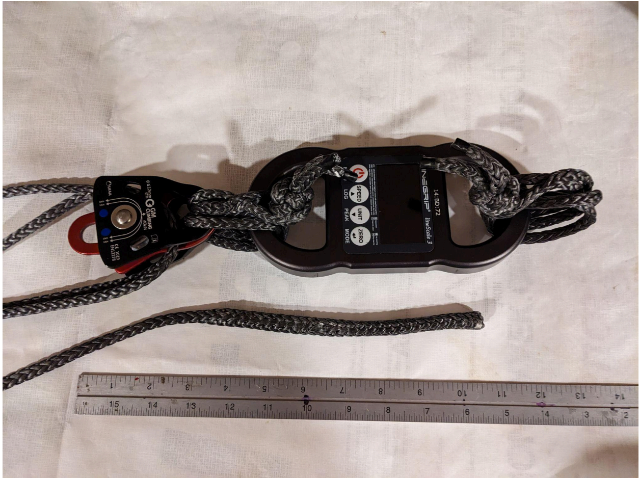
Fig: connecting the Linescale to the pulley as compact as possible by double wrapping the soft shackles
